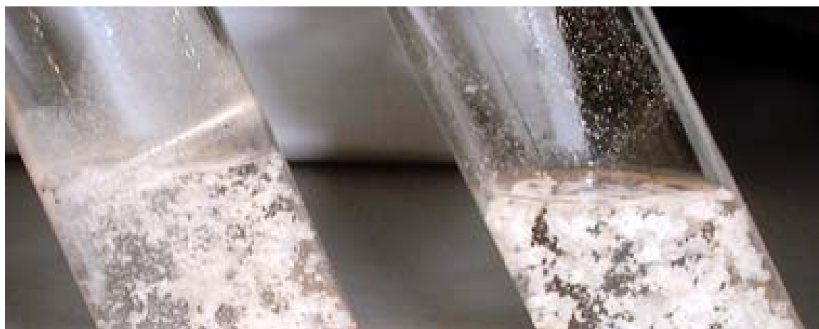
Fig 2 Appearance of the fill line zone on PET vials with no coating (left) and dual-layer coating (right) after exposure to formulation for 1 week
