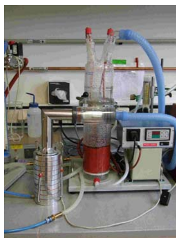
Figure 3: Connection between ACI and humidifier
