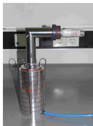
Figure 1: USP Apparatus 1 with fitted Respimat® Soft Mist™ inhaler
