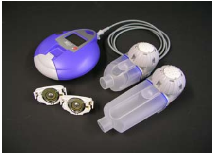
Fig. 1: Appearance of customised eFlow ® electronic nebulizer configurations. The base unit is shown in the left side of the picture and the handset configurations at the right side of the picture. Extension of the mixing chamber from about 48 ml (L) to 94 ml (XL) increases the delivered dose from 69.8% to 76.4% when using an atomising head class 30 and reduces in parallel the expelled fraction from 9.3% to 4.3% [7].
