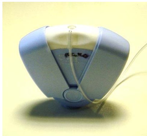
Figure 1. Prohaler DPI (Valois), showing tubing used to record pressure at mouthpiece.
